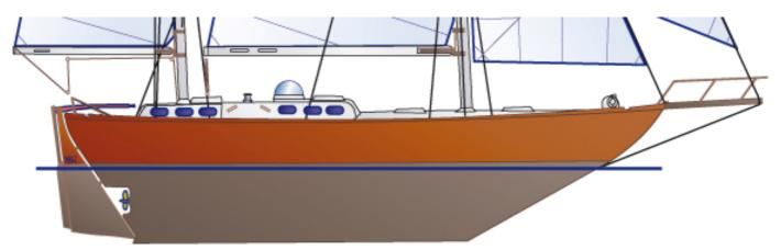
Exemple of rudder separated from the keel (here with a classique keel, ie with garboard strake)
