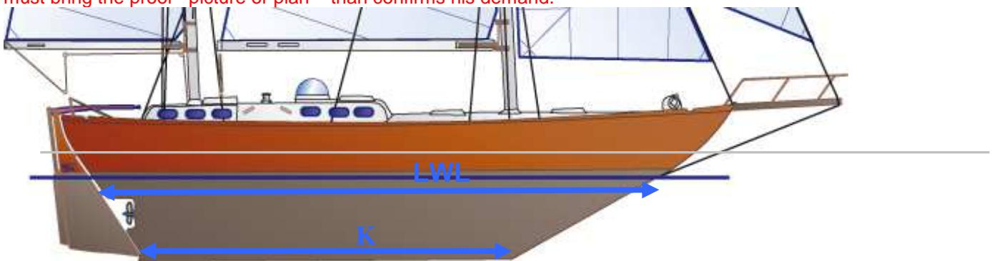
Exemple of rudder separated from the keel (here with a classic keel, ie with garboard strake)
