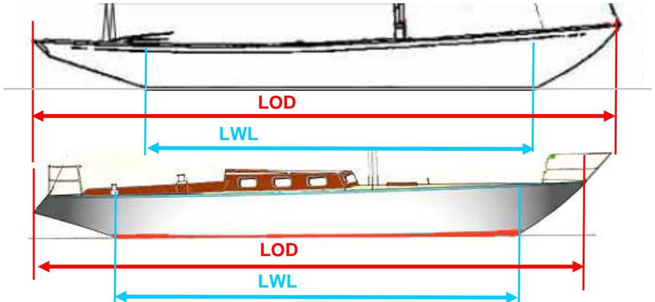
Long keel : is considered as a long keel when, as in the below example, the ratio  $K/LWL$  is higher than 60%. The owner must bring the proof -picture or plan - than confirms his demand.
