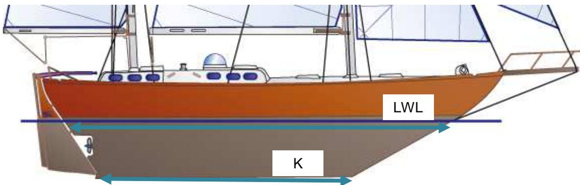
Example of rudder separated from the keel (here with a classic keel, ie with garboard strake)
